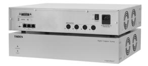
The maximum capacity of HCS-8300M series CMU is 60 contribution units. If extra contribution units are needed, HCS-8300ME/FS or HCS-8300ME Congress Extension Main Unit(s) must be added. The outlet connectors of both are identical. Each HCS-8300ME/FS or HCS-8300ME has two EXTENSION IN interfaces used to connect HCS-8300M series CMU or a preceding Congress Extension Main Unit, and an EXTENSION OUT interface for the next Congress Extension Main Unit.
